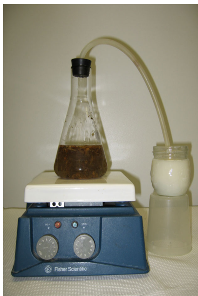
Figure 1. Setup for preparing milk sample with off flavor of feed
